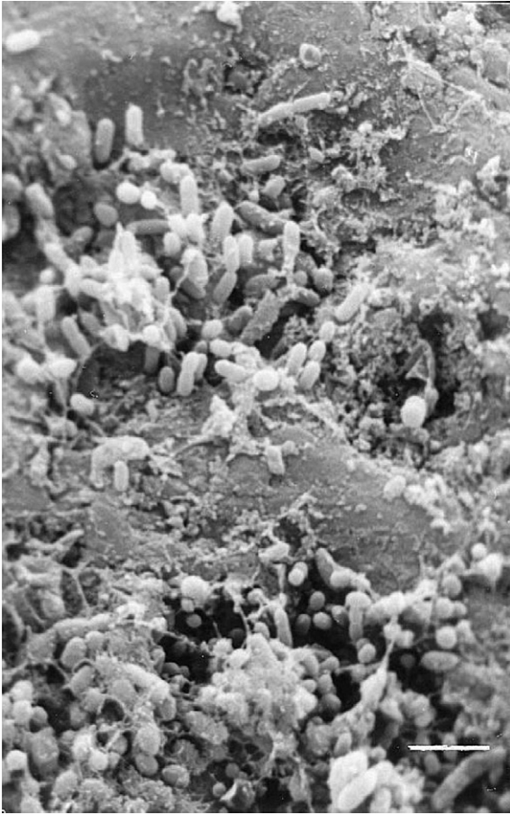
Fig. 3. Microbial colonies on granular activated carbon three days after incubation. Growth during early stages of colonization occurs primarily in rough areas and within cavities (from [90]).
