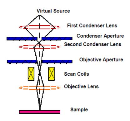
1) The "Virtual Source" at the top represents the electron gun, producing a stream of monochromatic electrons.
